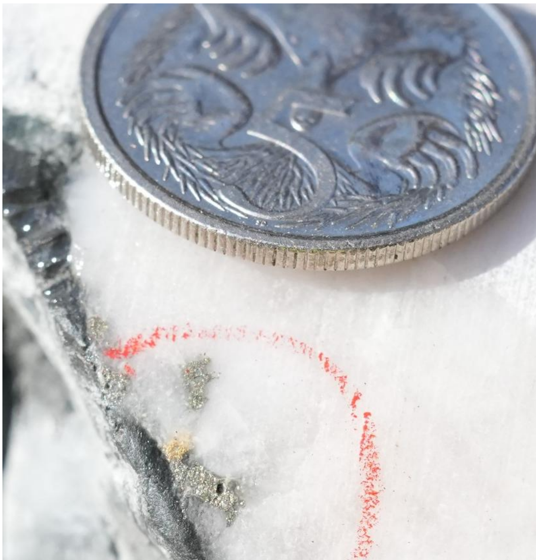
Figure 3 Trace of visible gold with pyrite in BMDD010 at 184.5m at the Morning Glory Zone
