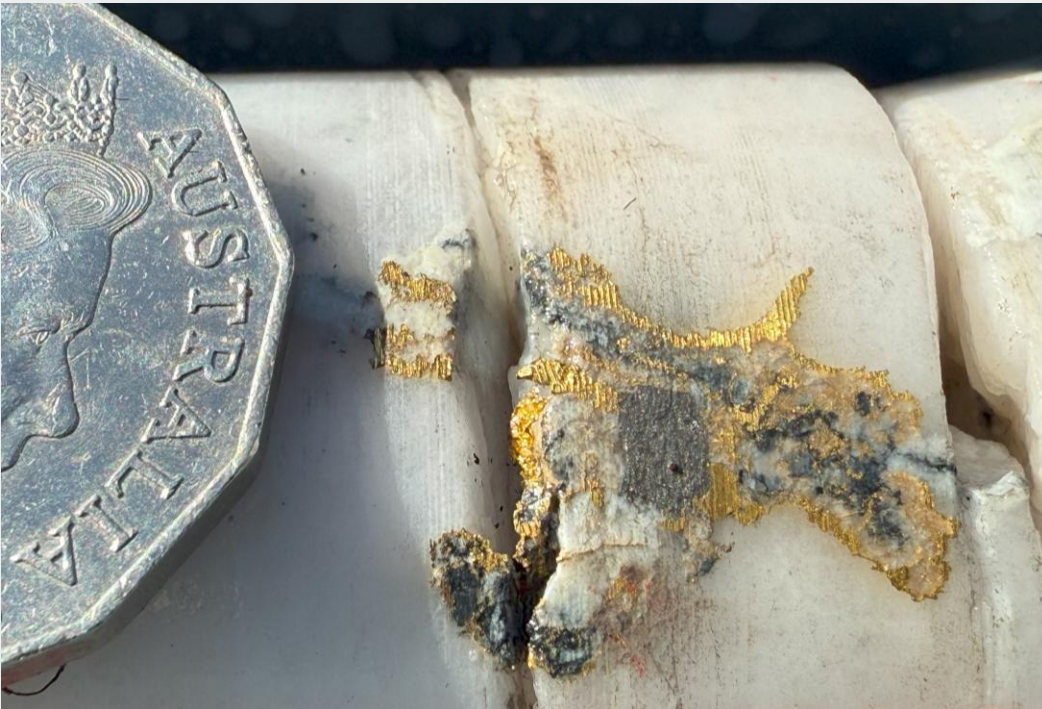
BMDD001W1 – visible gold at 544.6m in intercept 1.2m @ 543g/t Au from 544.2m 1
