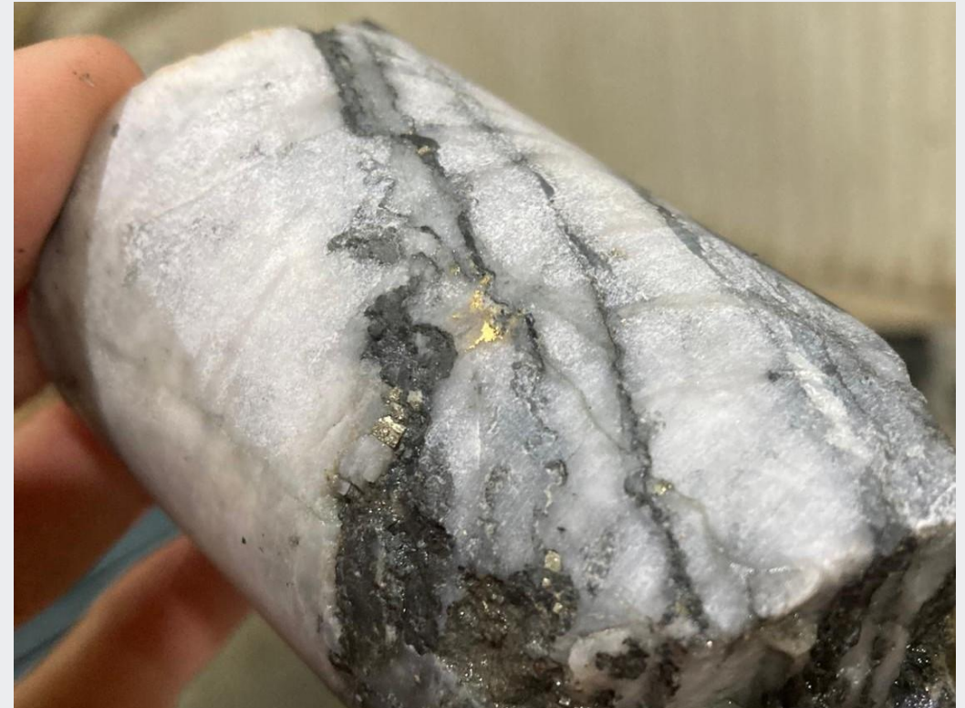
BMDD001W6 – visible gold at 832.7m in NQ core (47.6mm diameter) in intercept 6.5m @ 33g/t Au from 832m 1
