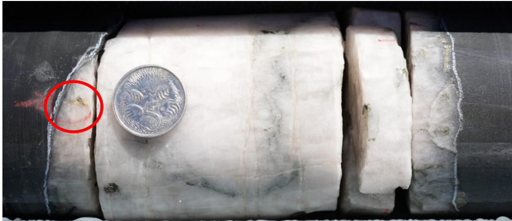
Figure 10 BMDD003 with visible gold (red circle) in an extensional quartz vein with pyrite near the vein margins at 605.6m
