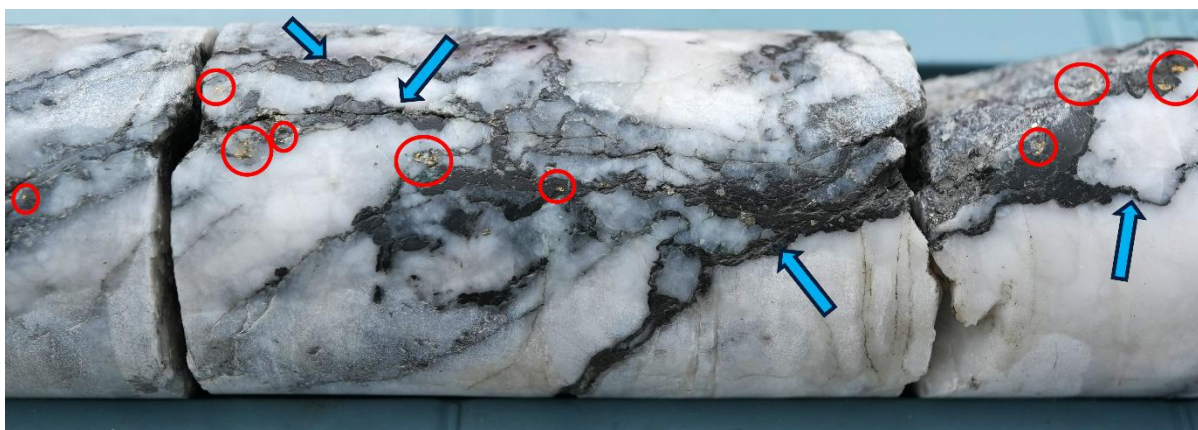
Figure 7 BMDD001W6 showing visible gold (red circles) and stylolites (blue arrows) in the NQ core (47.6mm diameter) from 832.7 to 832.9m
