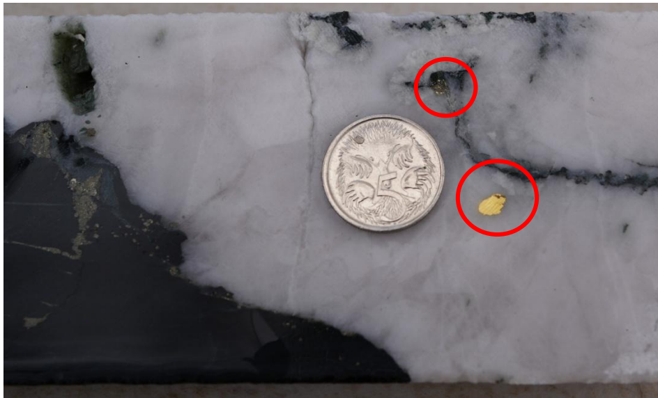
Figure 12 BMDD003 showing visible gold (red circles) on the cut surface of the stylolitic quartz carbonate vein at 607.6m
