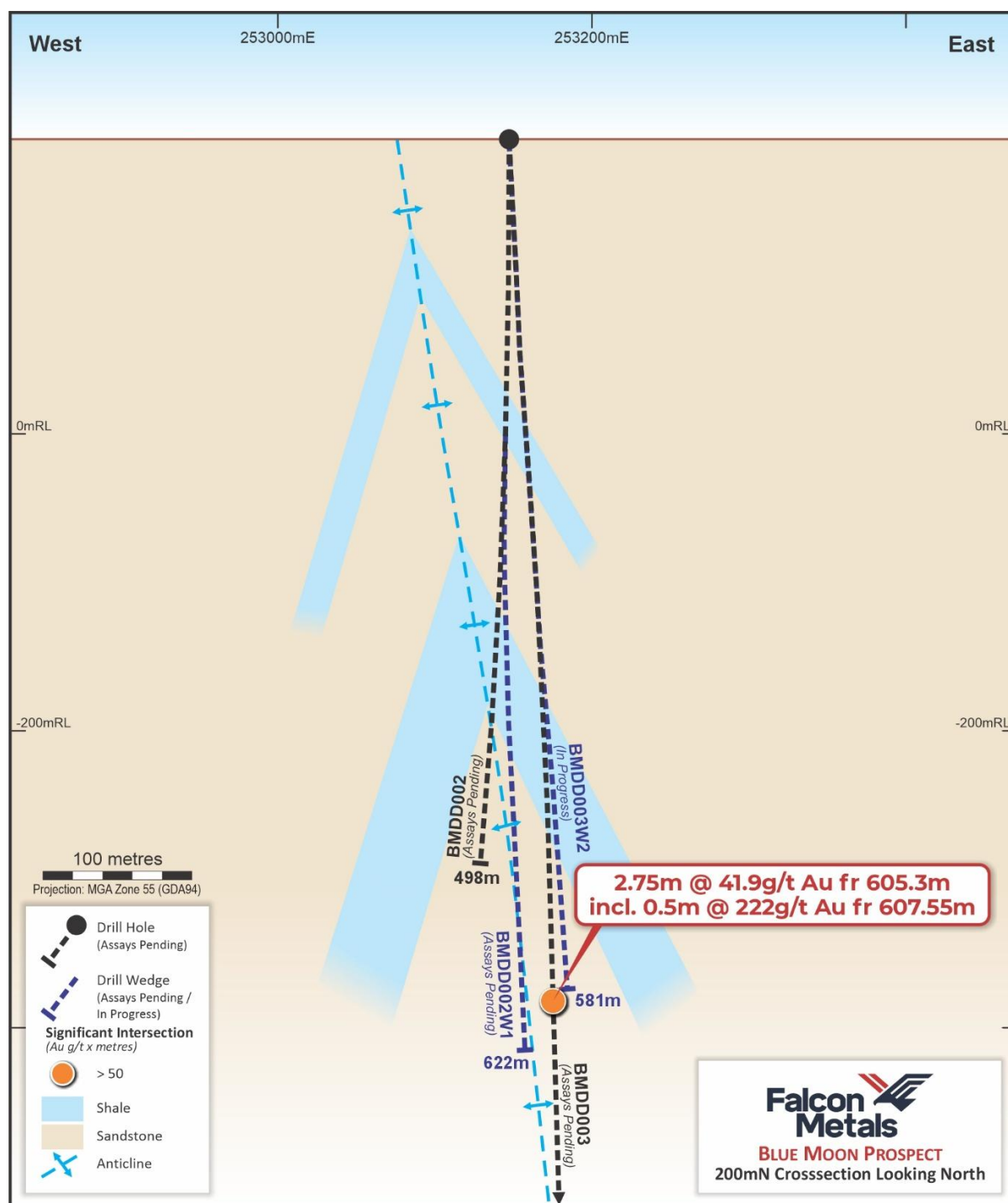
Figure 9 Cross section of BMDD002 and BMDD003
