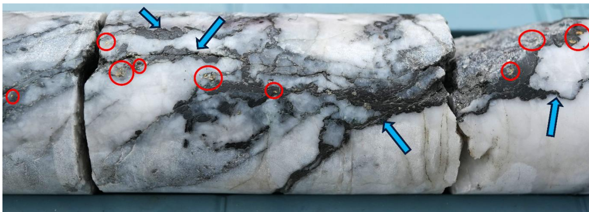
Figure 7 BMDD001W6 showing visible gold (red circles) and stylolites (blue arrows) in the NQ2 core (50.6mm diameter) from 832.7 to 832.9m
