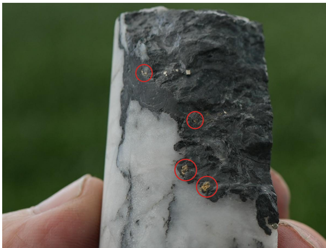
Figure 11 Visible gold in NQ core (47.6mm diameter) in BMDD001W6 at 832.9m
