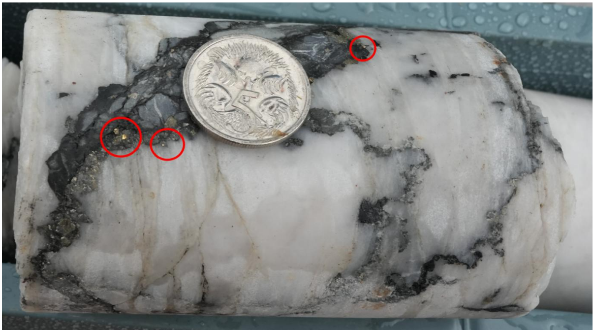
Figure 8 BMDD001W6 showing visible gold (red circles) in the NQ core (47.6mm diameter) from 834.8m
