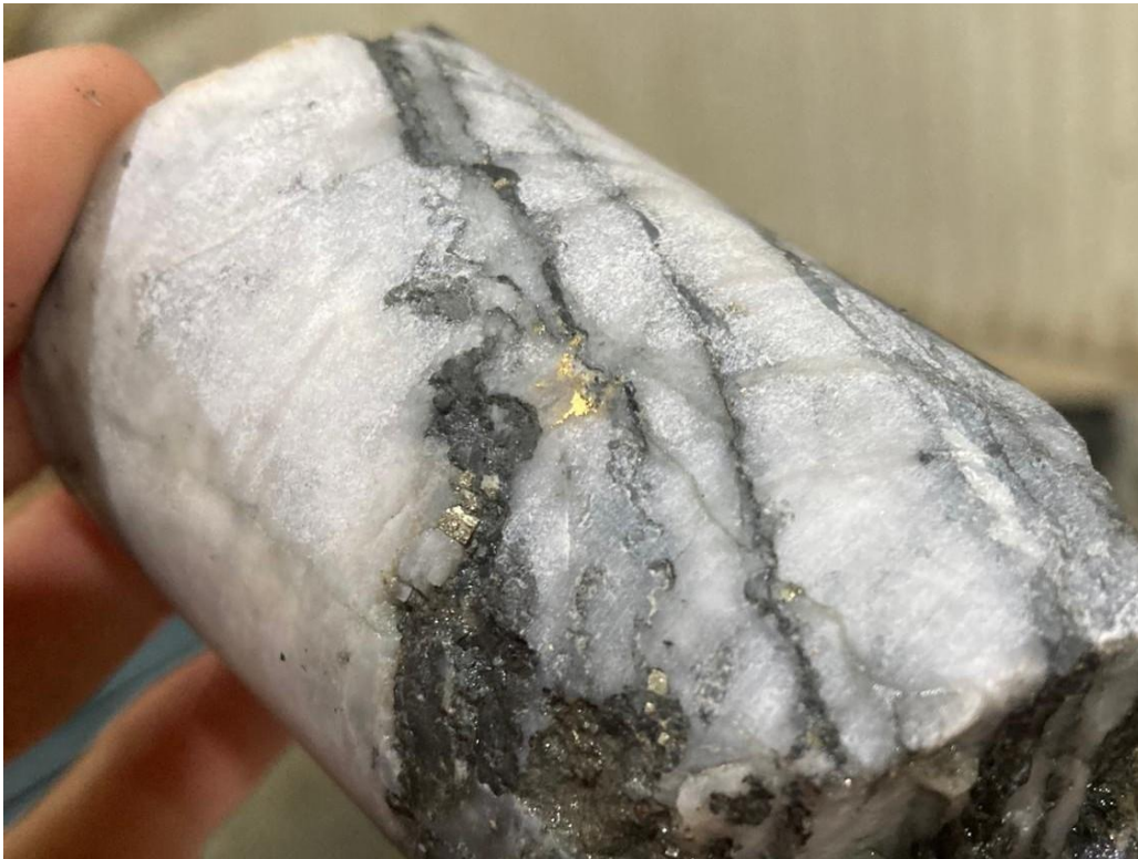
Figure 1 Visible gold from BMDD001W6 at 832.7m in NQ core (47.6mm diameter)
