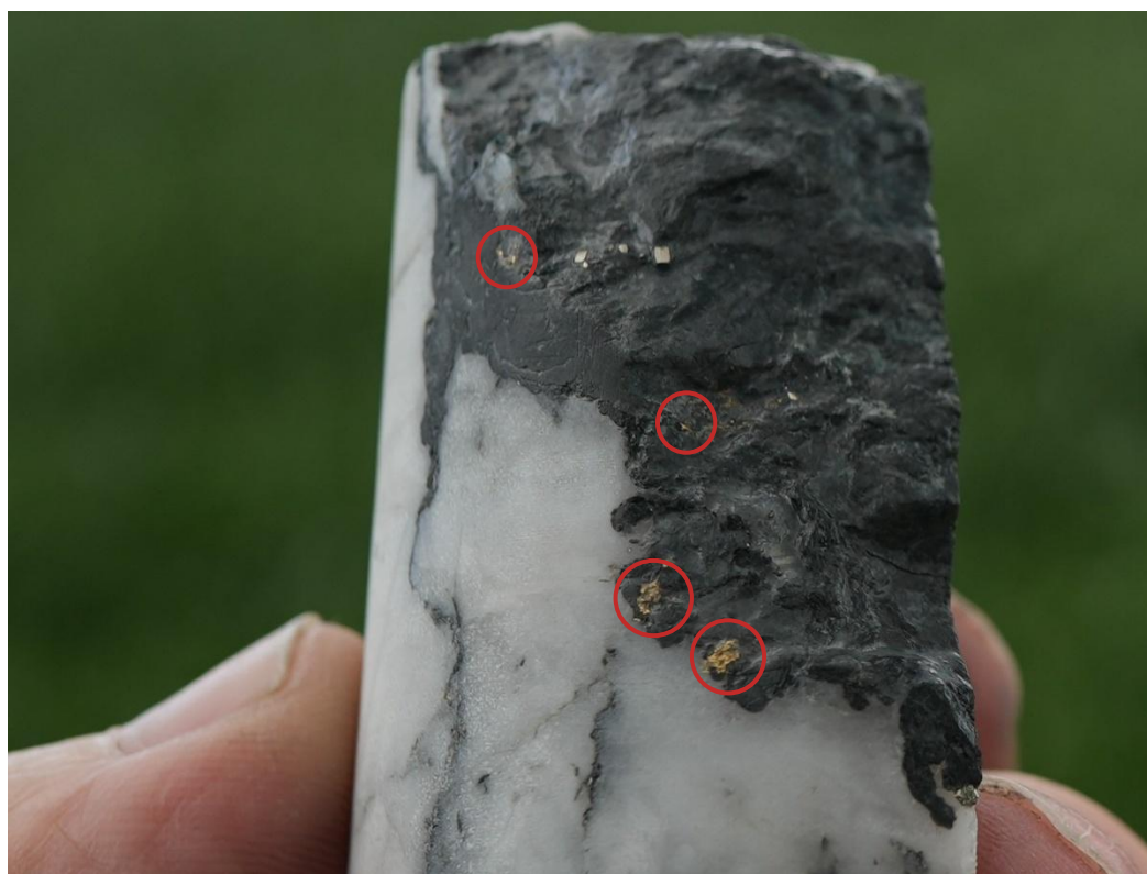
Figure 10 Visible gold in NQ core (47.6mm diameter) in BMDD001W6 at 832.9m
