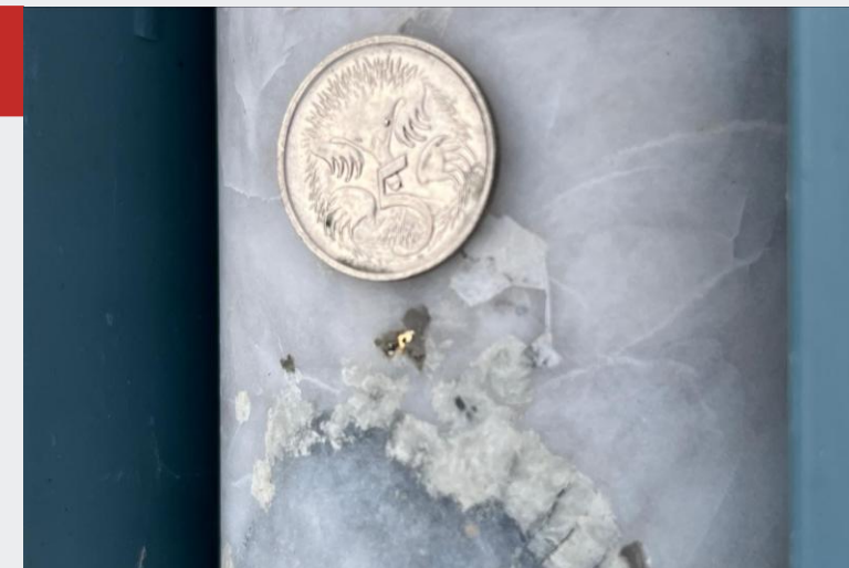
Visible gold in BMDD001 from 600.2m depth
