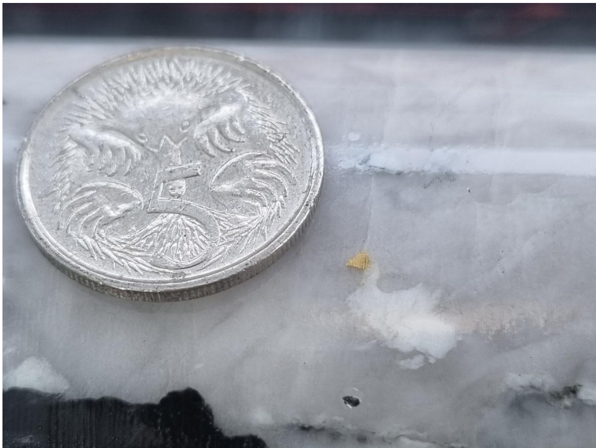
Figure 9 Close up of visible gold at 773.1m in the NQ core
