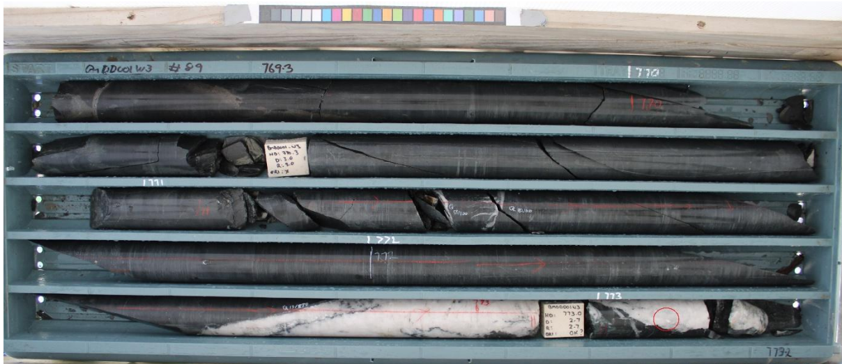
Figure 8 Laminated quartz vein with trace of visible gold at T773
