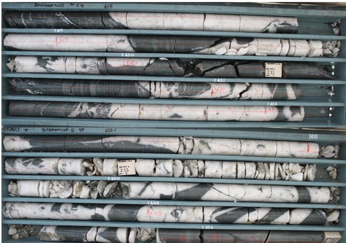
Figure 10 Saddle/neck reef with spur veins in BMDD001W3
