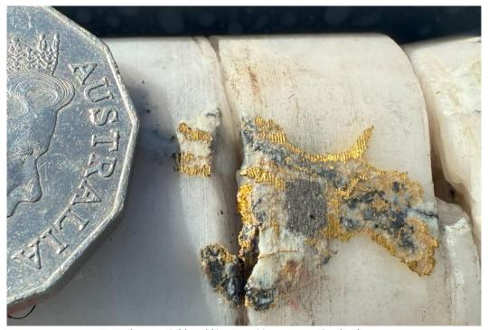
Figure 1 Visible gold in BMDD001W1 at 544.6m depth
