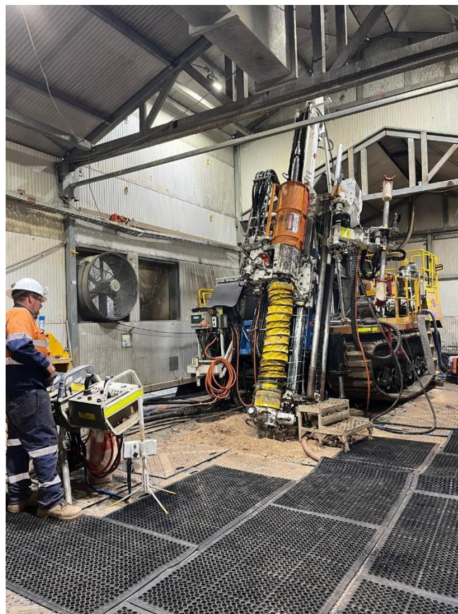
Figure 1 Diamond drill rig operating inside the acoustic shed at the Blue Moon Target
