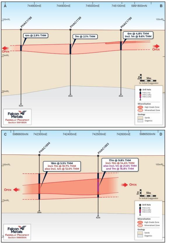
Figure 8 Cross-sections A-B and C-D through the Farrelly Prospect showing holes with results received
