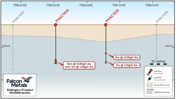
Figure 5 Cross Section showing results at Eddington
