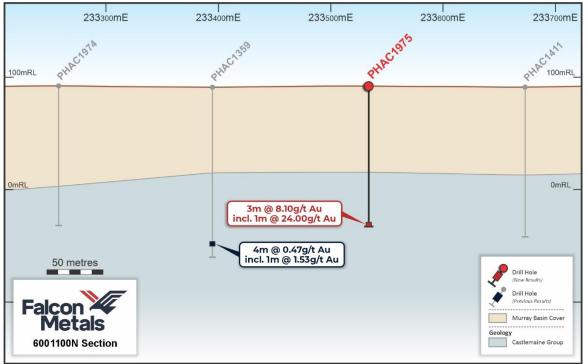
Figure 3 Cross Section showing high-grade result in PHAC1975
