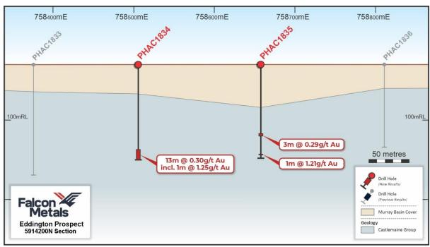
Figure 5 Cross Section showing results at Eddington
