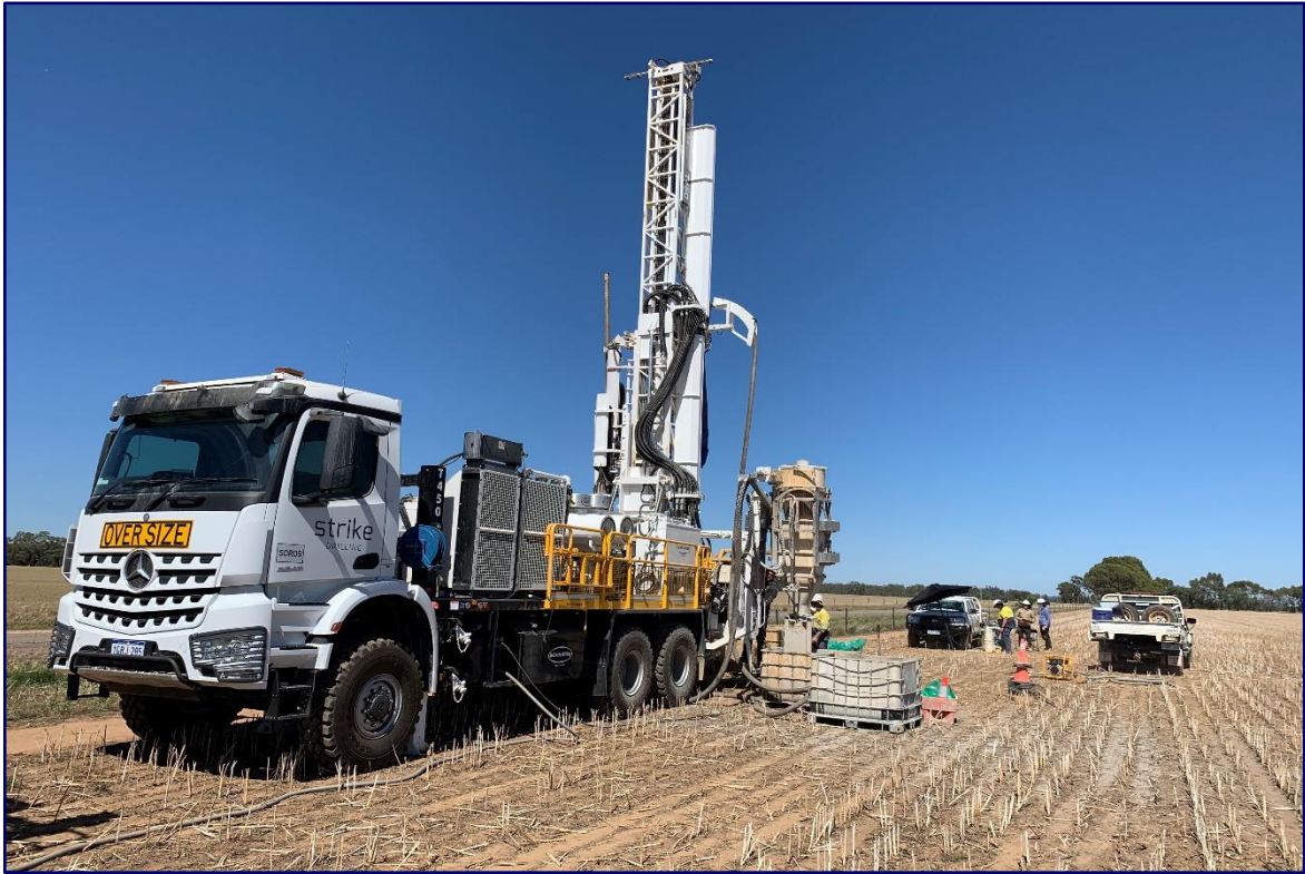
Figure 3 Falcon drilling set up (Aircore - Strike)
