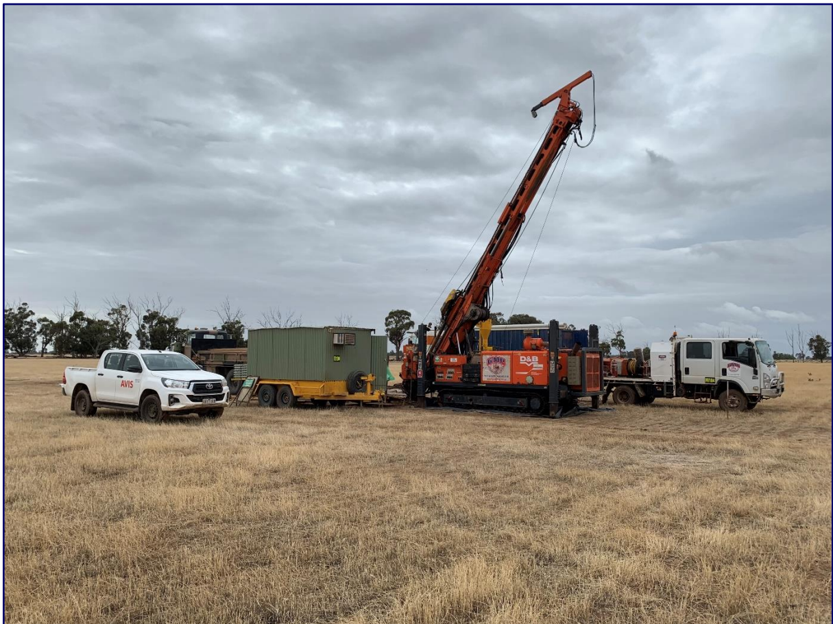
Figure 5 Falcon drilling set up (Diamond – GMP Drilling)
